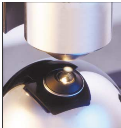
surface texture (RMS) to sub-angstrom levels can be measured on super-polished optical components
